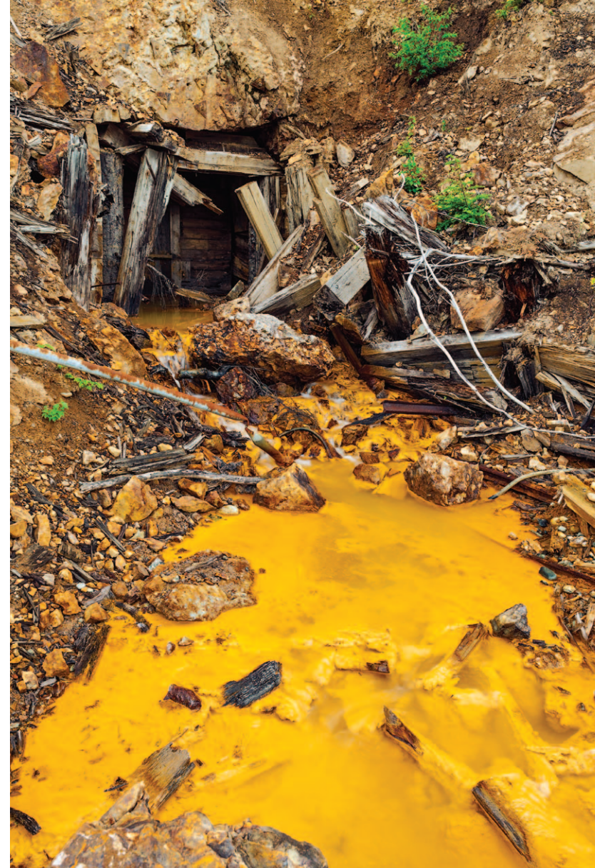
Acid drainage leaves one of several adits for the Tulsequah Chief Mine in British Columbia, Canada. The Tulsequah Chief Mine contains ore deposits of copper, lead, zinc, gold, and silver and operated from 1951 to 1957. The site is currently under development by Chieftain Metals Inc.
